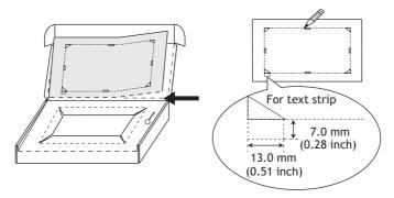
3. Secure the operator terminal in position, using all the fastening holes and the provided brackets and screws:
